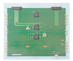
Full-view photo of the developed optical PCB ( size: 300mm x 250mm, 10 layers of FR4) Four channels of optical waveguide were formed between A and B, with overall length of 32cm. Low transmission loss of below 4 dB was realized ( wave length 850 nm).
